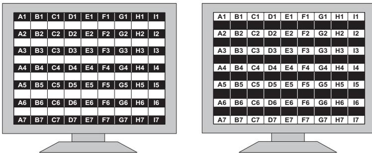
**Figure 2. The measurement setup. Two screens were necessary as each screen position had to be measured in a dark and a bright version.**
