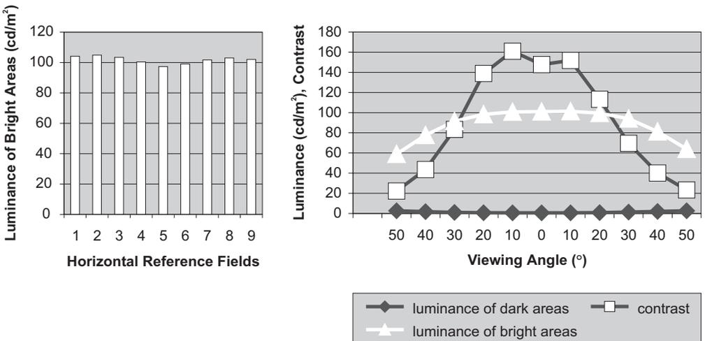
**Figure 4.** Left: A standard view the 63 luminance values (averaged over vertical rows). Right: A bystander view with luminance values (dark-bright) and contrast due to different viewing angles.
