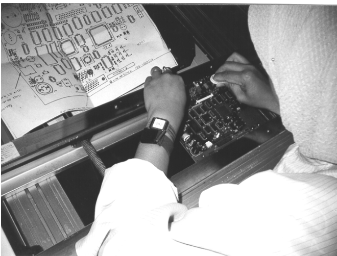
Figure 3. Finger work aids were used for pressing sharp top-edged and tight components.
