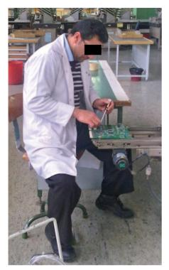
Figure 1. Board assembly unit (BAU): a worker is assembling a board. His neck and back are bent and in awkward static posture.
