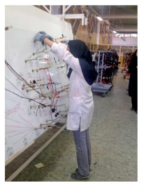
Figure 2. Cable assembly unit (CABLE): a worker is weaving wire standing on her tiptoes. The posture of her shoulders and upper arms is considerably deviated from neutral.
