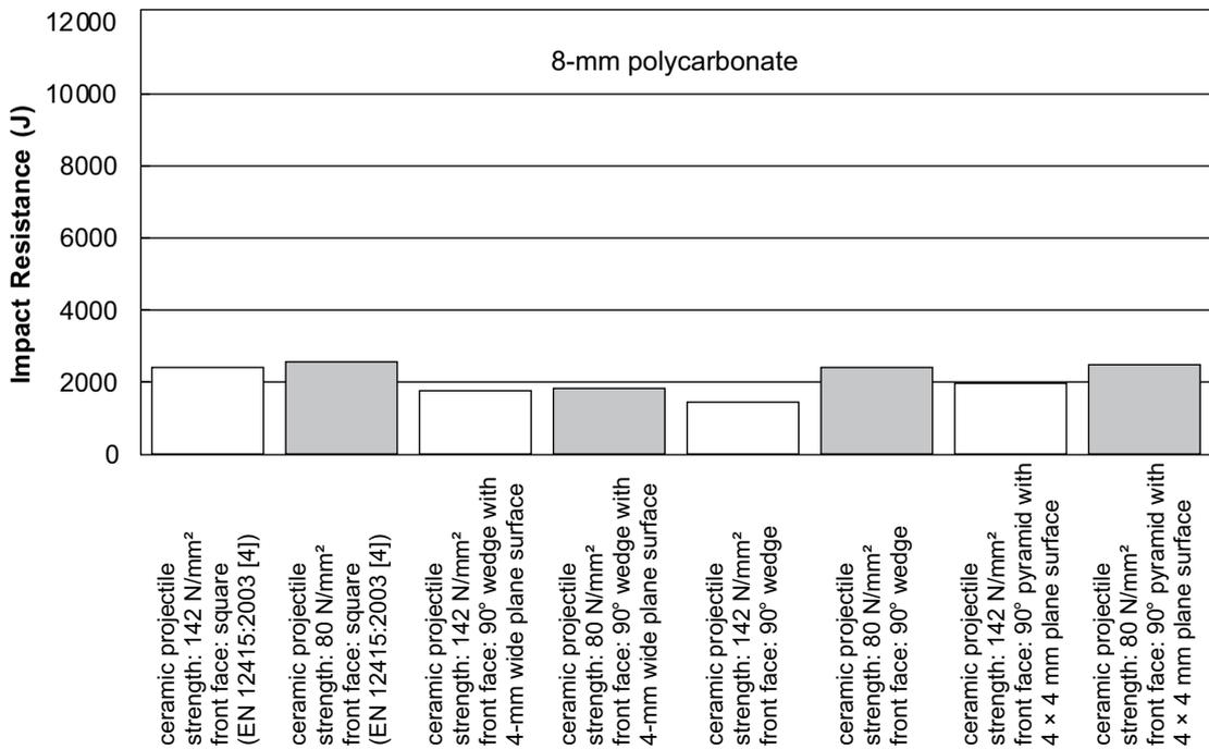
Figure 10. Impact resistance of 8-mm polycarbonate using ceramic projectiles (diameter: 40 mm, mass: 1250 g) with different front faces.
