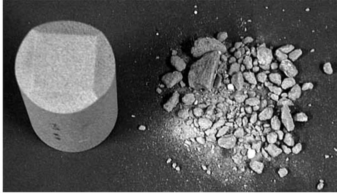
**Figure 7. Ceramic projectile (strength: 80 N/mm<sup>2</sup>) with front face in accordance with Standard No. EN 12415:2003 [4] before impact (left) and after impact (right), projectile energy: 9303 J.**
