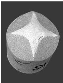
**Figure 8. Ceramic projectile (strength: 80 N/mm<sup>2</sup>) with 90° pyramidal front face and 4 × 4 mm plane surface after impact on steel sheet, projectile energy: 1381 J.**
