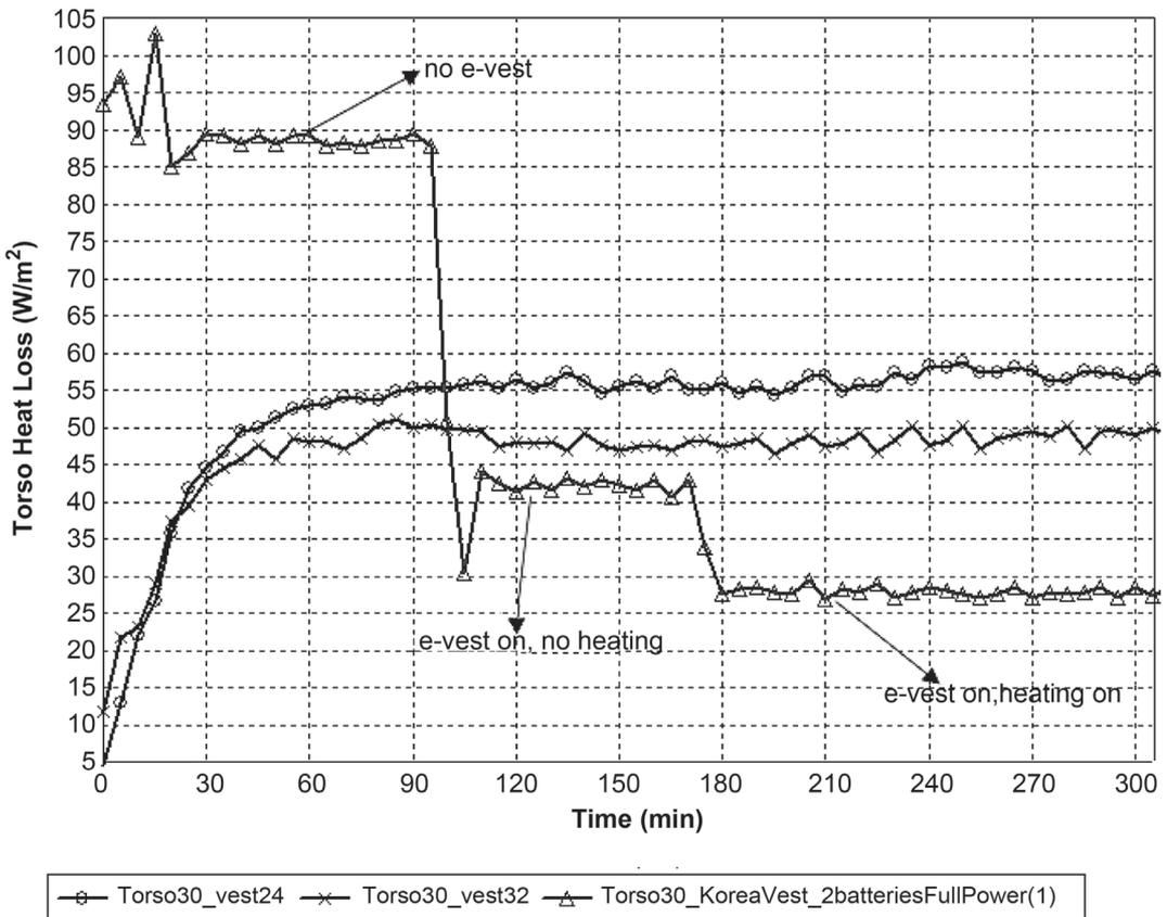
Figure 3. Manikin torso heat losses for phase change material (PCM) vests and electrical heating vest [34]. Notes. PCM vests worn over manikin stretch coverall,  $T_{manikin} = 30 \text{ }^\circ\text{C}$ ,  $T_a = -4 \text{ }^\circ\text{C}$ ,  $V_a = 0.4 \text{ m/s}$ .
