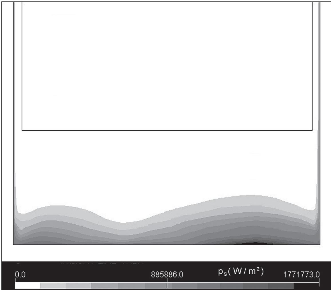
Figure 9. Distribution of surface density of power loss  $p_s$  ( $W/m^2$ ) (corresponding to discretized surface elements) in the bottom part of the frame for the system in Figure 7, at phase current of  $I_h = 4000$  A (the bottom rod of the frame is magnified).
