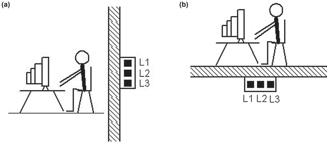
Figure 6. Examples of unsuitable arrangements of workstands near busducts: (a) interaction through a wall, (b) interaction through a floor. Notes. L1, L2, L3—phase conductors.
