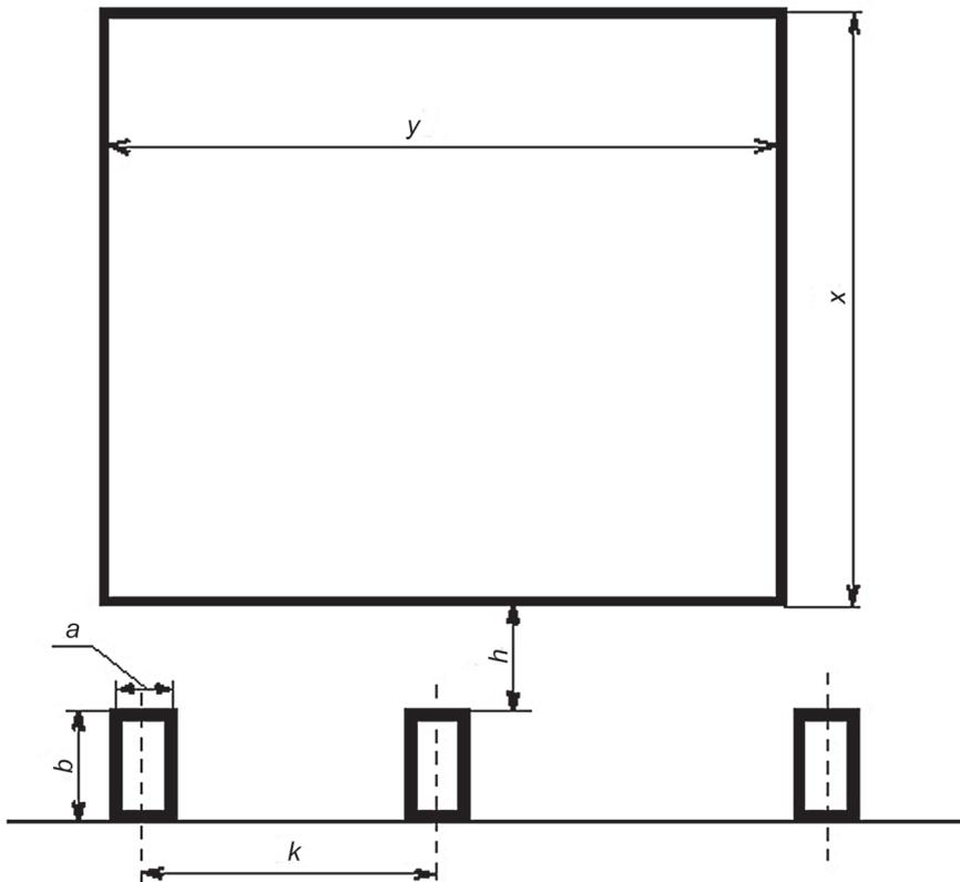
Figure 7. Arrangement of a ferromagnetic frame located above a busduct. Notes.  $a$ ,  $b$ —dimensions of conductors,  $k$ —distance between axes of conductors,  $h$ —distance between busduct and frame.
