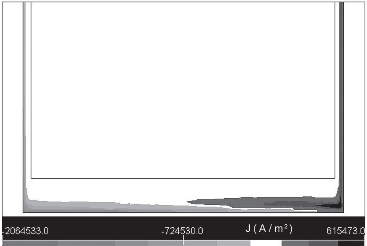
**Figure 8.** Distribution of current density  $J$  ( $\text{A}/\text{m}^2$ ) induced in the bottom part of the frame of the system shown in Figure 7, at phase current of  $I_n = 4000$  A (the bottom rod of the frame is magnified).
