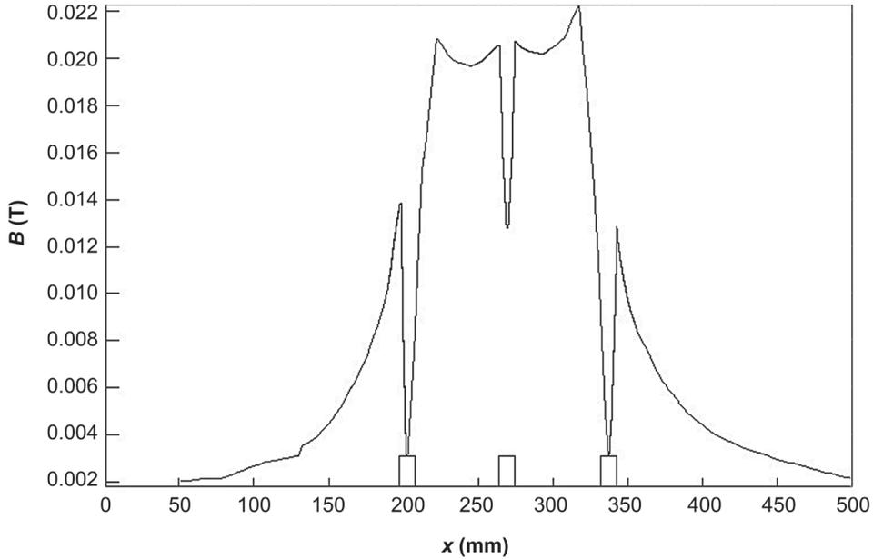
**Figure 2.** Distribution of magnetic flux density  $B$  (T) on the  $x$  axis of the phase conductors for the system in Figure 1b, with phase current of  $I_n = 1250$  A and the distance between the axes of the conductors  $k = 62$  mm. Notes.  $a, b$ —dimensions of the conductors.
