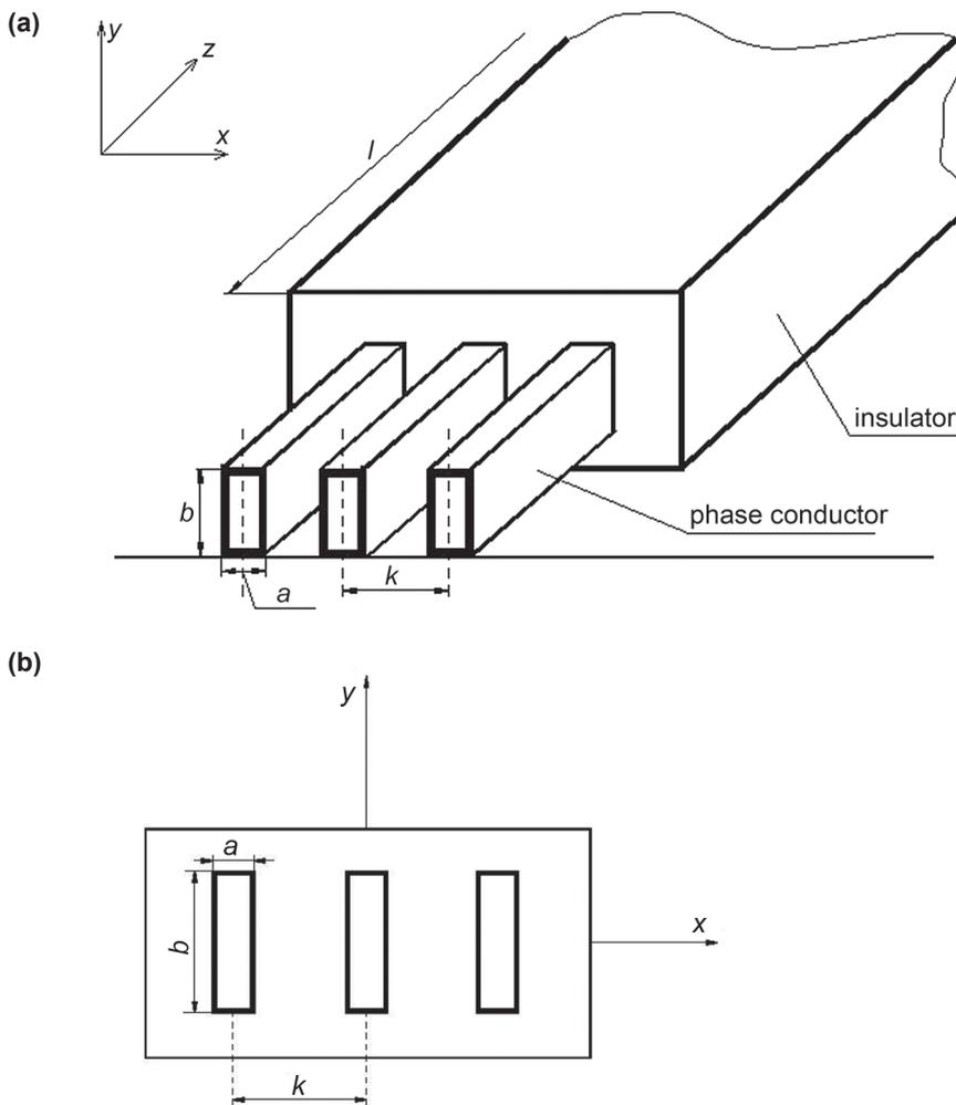
**Figure 1. Geometry of two system: (a) configuration of a busduct, (b) a busduct in a two-dimensional system (cross-section).** Notes.  $a$ ,  $b$ —dimensions of conductors,  $k$ —distance between axes of conductors.
