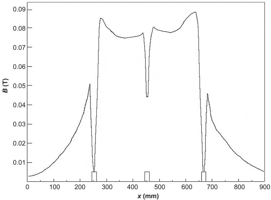
**Figure 3.** Distribution of magnetic flux density  $B$  (T) on the  $x$  axis of the phase conductors for the system in Figure 1b, with phase current of  $I_n = 4000$  A and the distance between the axes of the conductors  $k = 212$  mm.
