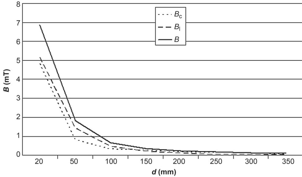
Figure 4. Dependence of magnetic flux density  $B$  (mT), longitudinal  $B_l$  (mT) and cross  $B_c$  (mT) components of the magnetic flux density vector as functions of the distance from the busduct  $d$  (mm).
