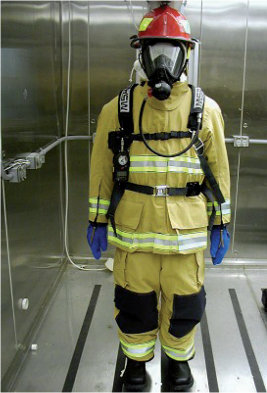
Figure 13. Sweating manikin test of deployed prototype.
