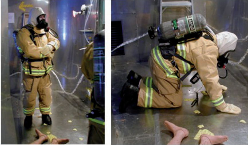
Figure 12. Evaluation of chemical and biological (CB) turnout prototype in man-in-stimulant test (MIST).
