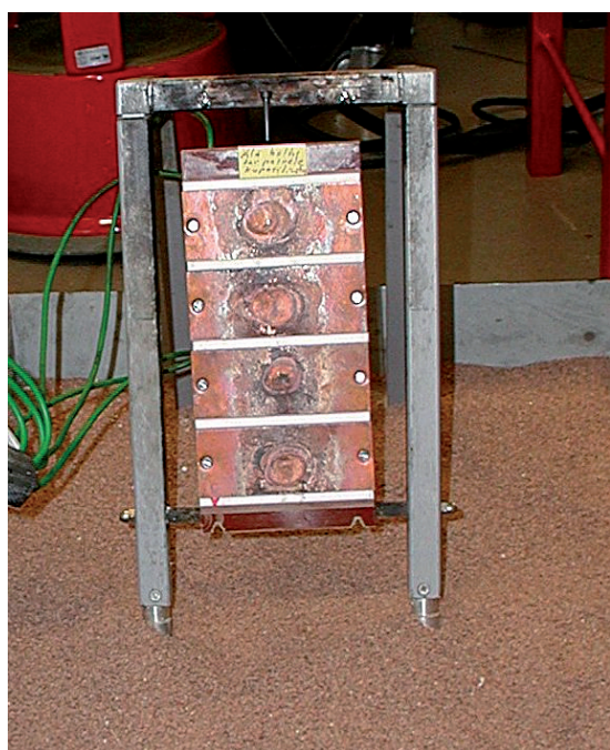
Figure 4. Copper-coated K-type thermometer for temperature measurements.
