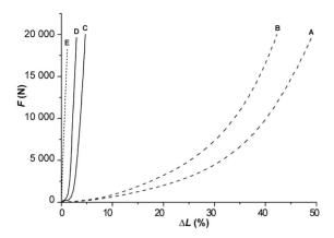
Figure 3. Examples of tension-elongation characteristics of ropes. *Notes.* A—14-mm diameter three-strand polyamide rope, B—18-mm diameter three-strand polyamide rope, C—10-mm diameter aramid rope, D—12-mm diameter aramid rope, E—8-mm diameter steel wire rope.
