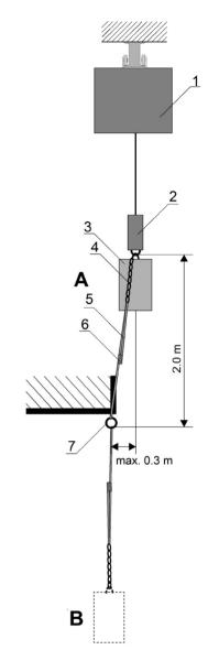
Figure 6. Dynamic strength test for lanyards (according to EN 364:1992) [5]. Notes. A situation before the test, B—situation after fall arrest, 1—power winch for lifting and lowering test mass, 2—quick release device, 3—test mass of 100 kg, 4—chain, 5—lanyard, 6—length adjuster of a lanyard, 7—anchor point.
