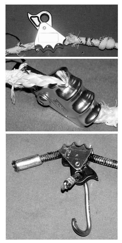
Figure 10. Examples of damage to ropes, length adjusters and connectors.
