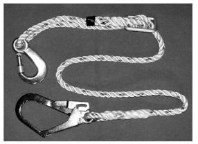
Figure 2. Lanyard made of a 14-mm diameter three-strand polyamide rope.
