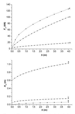
Figure 8. The results of a numerical simulation. Notes.  $F_m$ —maximum value of the force acting on the end of a lanyard,  $H_m$ —maximum value of the elongation of a lanyard; A—14-mm diameter three-strand polyamide rope, C—10-mm diameter aramid rope, E—8-mm diameter steel wire rope.
