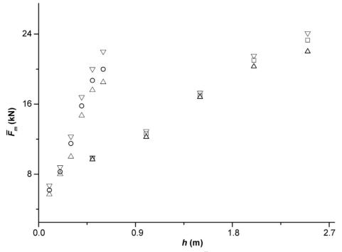
**Figure 9. Test results of adjustable lanyards.** *Notes.*  $\bigcirc -\overline{F}_m$  for lanyards made of steel wire rope with polyamide braid,  $\Box -\overline{F}_m$  for lanyards made of aramid rope,  $\bigtriangleup -\overline{F}_m \min, \bigtriangledown -\overline{F}_m \max$ .
