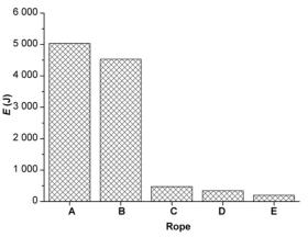
Figure 4. Energy (transformed into elongation) generating in a rope of the initial length of  $L_o = 2 \text{ m}$  a force of F = 20 kN. Notes. A—14-mm diameter three-strand polyamide rope, B—18-mm diameter three-strand polyamide rope, C—10-mm diameter aramid rope, D—12-mm diameter aramid rope. E—8-mm diameter steel wire rope.
