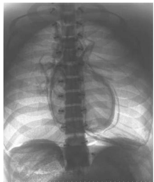
Figure 4. Ribcage and radiograph of AUSMAN surrogate. Notes. AUSMAN—a reusable mechanical surrogate developed by the Australian Department of Defense – Defense Science and Technology Organization (DSTO).
