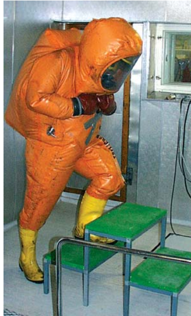
B. 2 min of ascending and descending stairs (height of footstep 27 cm) at one's own speed
