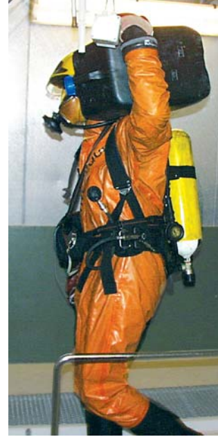
C. 2 min of carrying a 35-kg can on a treadmill, 3.5 km/hr, 1° grade
