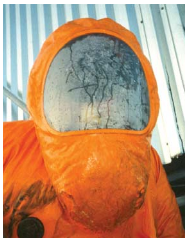
Figure 9. Misting of the visor was a problem while wearing an encapsulating chemical protective suits system.
